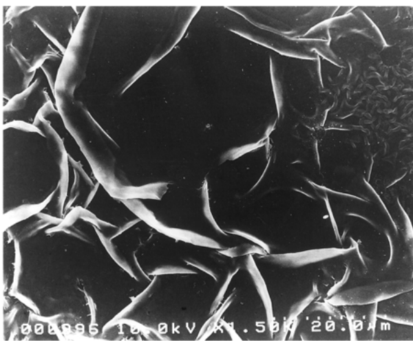
Figure 3 The SEM images of HA and BMP particles in HA. (a) A highly porous and sheet-like surface structure (central part), and a closely woven mesh-like structure (upper right) observed in HA. Original magnification is \times 1500 . (b) The meshwork structures composing a wall of pore (left side). Some particles of BMP (small arrow) and clumps of these particles (large arrow) are trapped by the meshwork of HA. Original magnification is \times 30000 .
